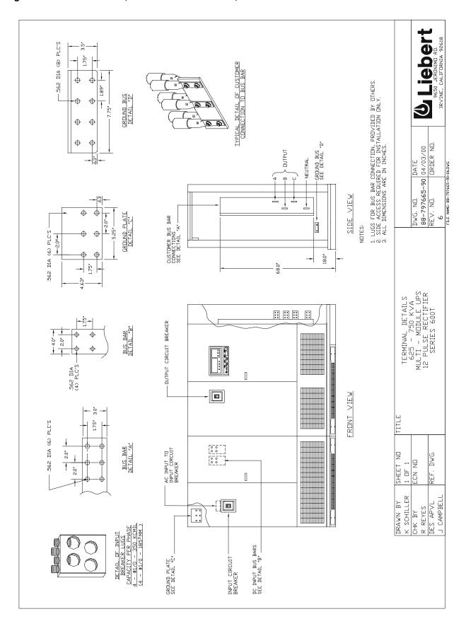
Figure 32 Terminal Details, 750 kVA/675 kW Std. and 750 kVA/600 kW with Optional Input Bus Bars
